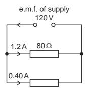
What is the internal resistance of the power supply?
